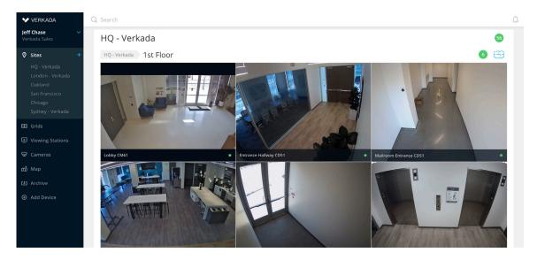
Command, Verkada's cloud-based management software, is designed to deliver simple access and management for all cameras and users across all sites from virtually anywhere in the world. From Command, users can set up new cameras, create new sites, manage settings, access live and archived footage, manage users, and access the advanced features powered by Verkada's edge-based analytics.
